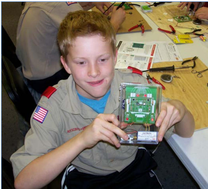
Scout Joel Martin shows the Electronics Merit Badge project he built in which transistors work as switches to blink LED lights. Photo courtesy of Carl Reichert
